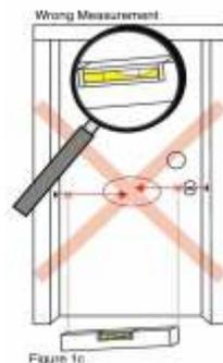
**Attention!** The right placement and function of the system involves that the two sensors will be located perfectly opposite to one another in a horizontal straight line without any object interjecting between them (e.g. doorknob, lock), so that the infra-red communication between them can be continuous
